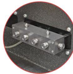
Multi-Port Manifold Outlet, allows multiple hose assemblies to be tested at the same time
