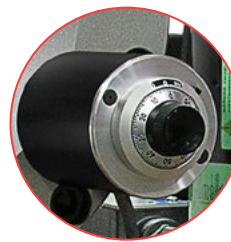
Dial Micrometer is fully adjustable provides speed, precision and repeatability
