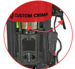
Retraction Stop limits ram retraction for quick repetitive crimps
