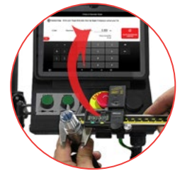
InfoCrimp™ controller supports bluetooth calipers to input crimp diameter measurements
