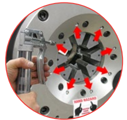
Easy grease maintenance through the 8 lubrication fittings
