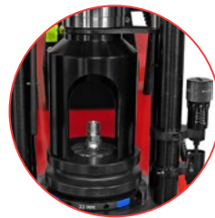
Electronic Stop Switch shuts the pump off when the crimp cycle is complete
