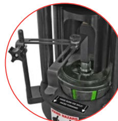
Coupling Stop makes repetitive crimps faster
