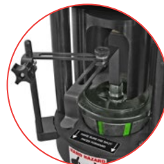
Coupling Stop makes repetitive crimps faster
