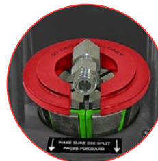
Ideal notched pressure plate when crimping 90 deg. fittings
