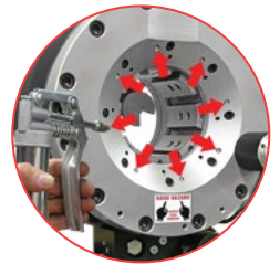
Easy grease maintenance through the 8 lubrication fittings
