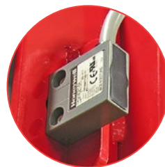
Safety Switch activates and drops pressure as soon as the lid is opened
