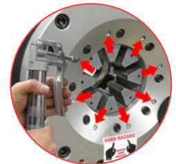
Easy grease maintenance through the 8 lubrication fittings
