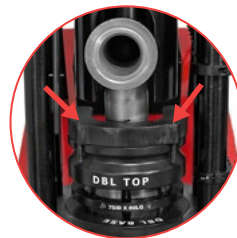
D200 Spacer Kit is ideal for crimping extra long elbow fittings
