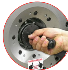
Quick change tool makes die changes a quick and simple process
