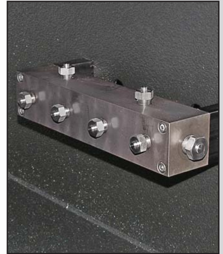
Multi-Port Manifold Outlet, allows multiple hose assemblies to be tested at the same time.
