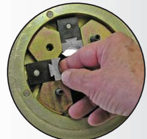
Quickly Exchangeable Dies: Remove the cover plate and slip another die finger into position.
