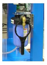
3) Another important task is to check the cleanliness of the supply water. Supply water can either be city water hook up or a reservoir system likely filled with a well or city water supply. While the filter bag and strainer will work to keep dirt and sentiment out of the water, they will not stop harmful chemicals or hard water.
