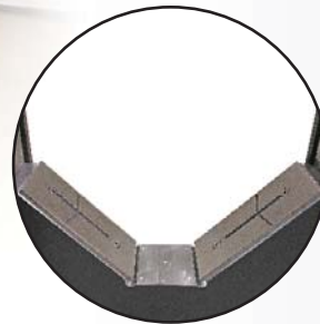
Inspection & Cleaning of the Master Die Wear Plates & Master Die Alignment Keys
