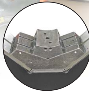
Inspection & Cleaning of the Master Die Carriers & Master Die Shoes
