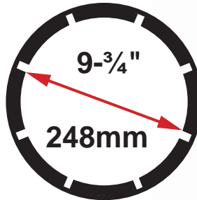
Max Head Opening W/O Dies: Can accommodate 4" 150 lbs SAE flange.
