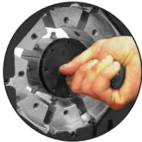
99mm Quick Change Tool (Included) P/N:102571
