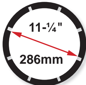
Max Head Opening W/O Dies: Can accommodate 6" 150 lbs SAE flange.
