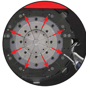
New Grease Applied on All Wear Surfaces
